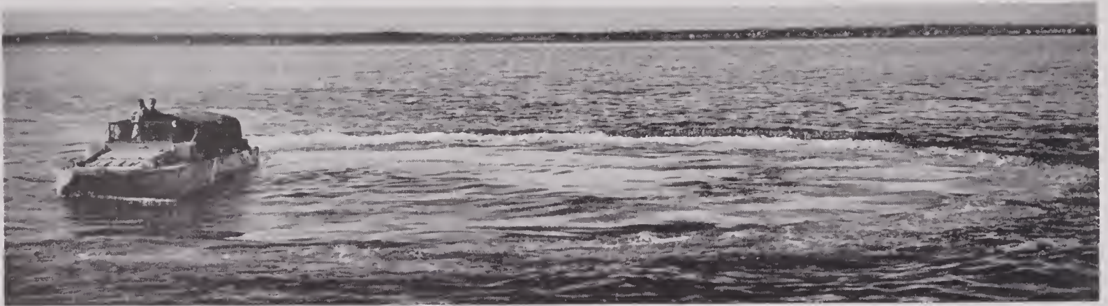
FIGURE 51. Minimum turning diameter in water is 75 to 110 feet for 1912 pilot model DUKW. 40 feet for production model shown here.
